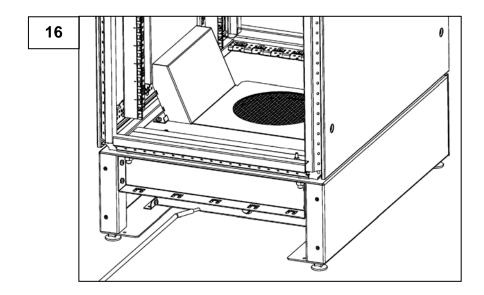
The condensate drain of the LHX 3 is situated at the bottom of the cabinet, close to the water connection points. To allow drainage of condensed water, remove the rubber cap and fit a hose (connecting pipe diameter 6 mm) to the condensate drain outlet (Figs. 15 and 16).
