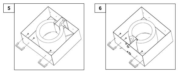
Next, loosen the screws on both handles and fit them to the opposite side of the heat exchanger facing outward (Figs. 5 and 6).
