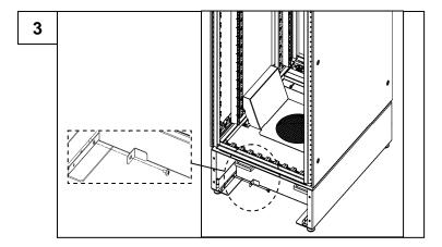
In order to change the water connection points from the rear to the front, first remove the heat exchanger cassette. Also remove the transport securing bracket (Fig. 3)
