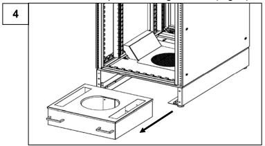
Now you can pull the heat-exchanger cassette out of the base unit (Fig. 4) and change the direction of water connection (select either from in front or from the rear).
